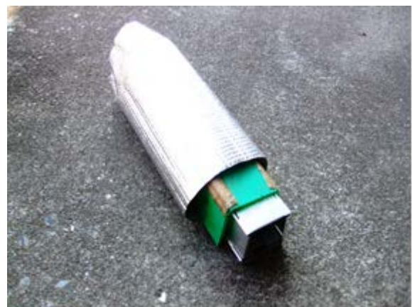
Fig.2. Heat insulation materials holding a trap.
